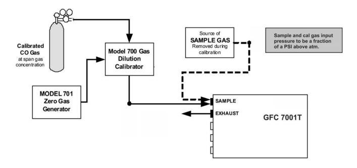
Figure 3-19: Pneumatic Connections-Basic Configuration-Using Gas Dilution Calibrator
